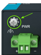
Figure 12: Grounding screw position
