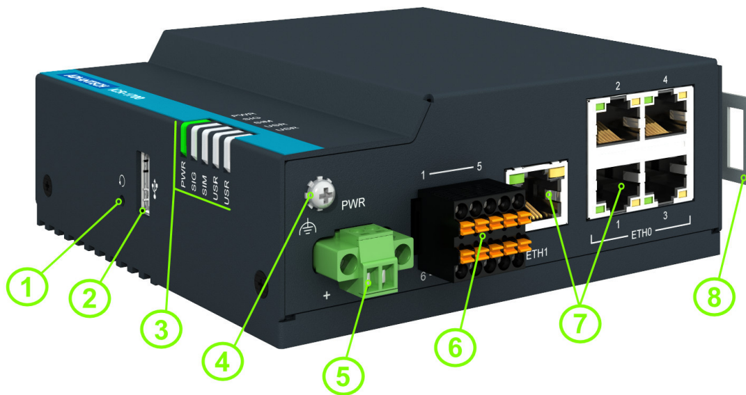
Figure 1: Router hardware overview – front view
