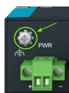
Figure 12: Grounding screw position
