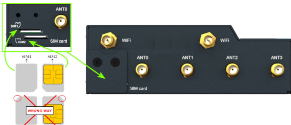
Figure 9: SIM card insertion
