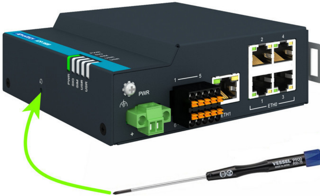
Figure 16: Resetting the router
