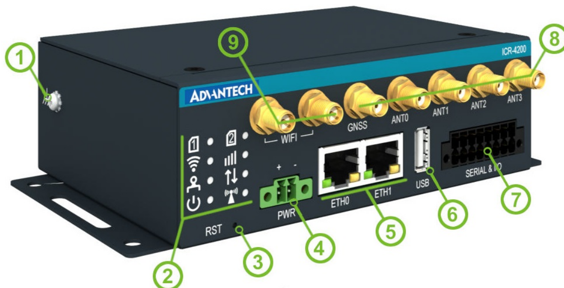
Figure 1: Router hardware overview – front view
