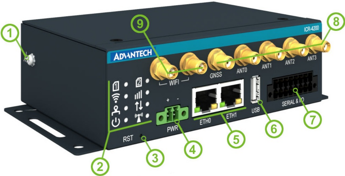
Figure 1: Router hardware overview – front view
