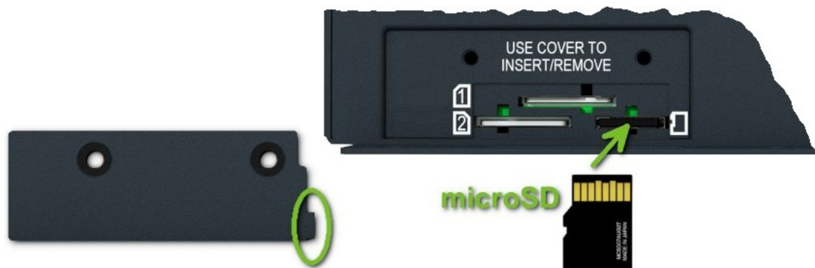
Figure 14: microSD card insertion
