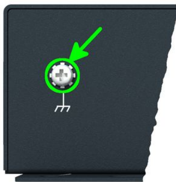
Figure 12: Grounding screw position
