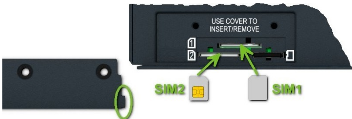
Figure 9: SIM card insertion
