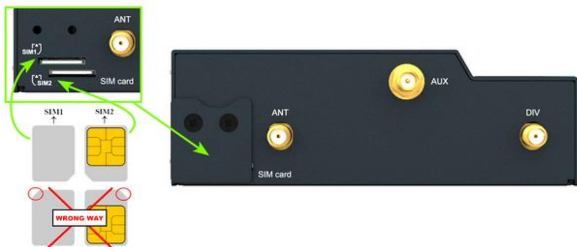
Figure 9: SIM card insertion
