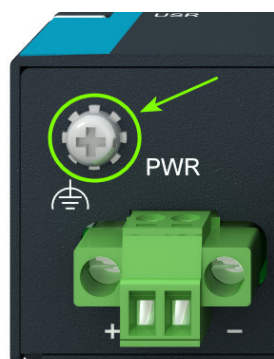
Figure 16: Position of the Grounding Screw
