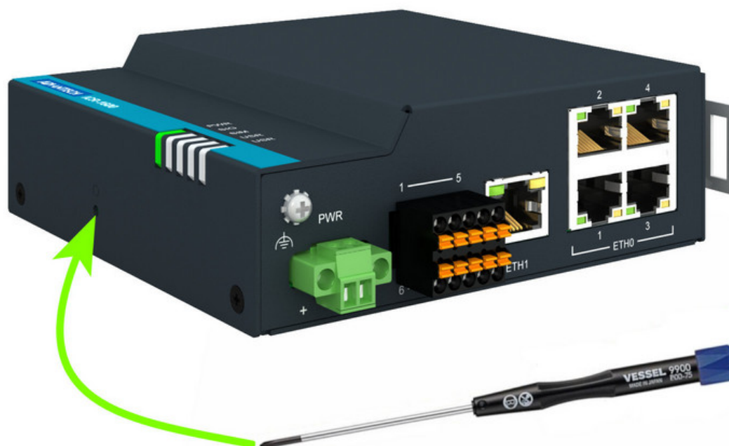
Figure 20: Resetting the Router
