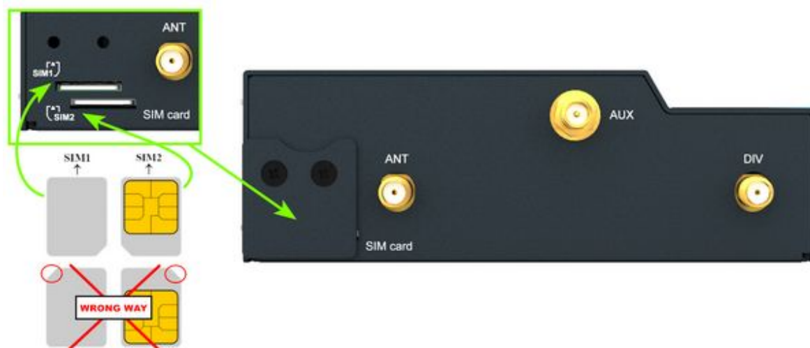
Figure 13: SIM Cards Insertion
