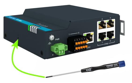
Figure 20: Resetting the Router
