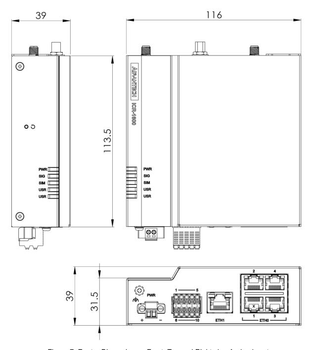
Figure 7: Router Dimensions – Front, Top and Right view for basic set
