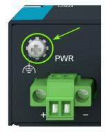
Figure 16: Position of the Grounding Screw
