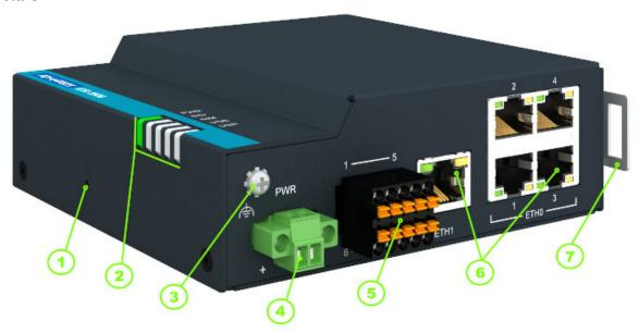
Figure 5: Router Hardware Overview - Front View
