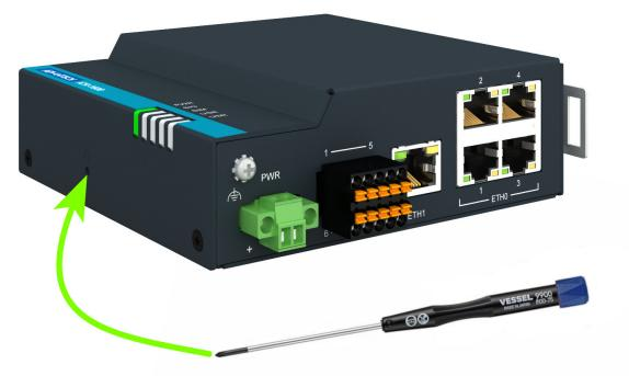
Figure 20: Resetting the Router
