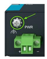
Figure 16: Position of the Grounding Screw
