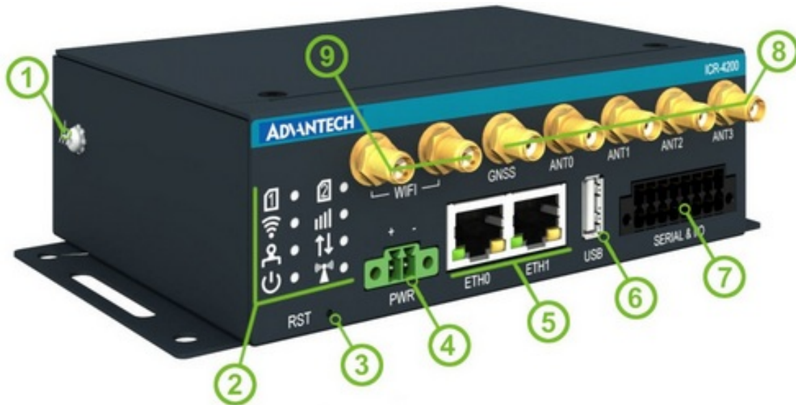
Figure 1: Router hardware overview – front view
