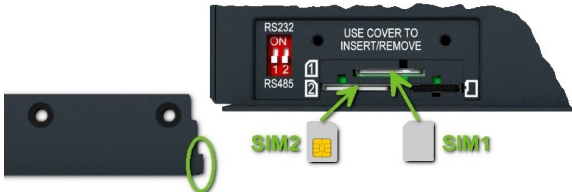
Figure 9: SIM card insertion
