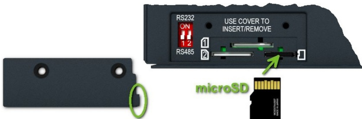
Figure 18: microSD card insertion
