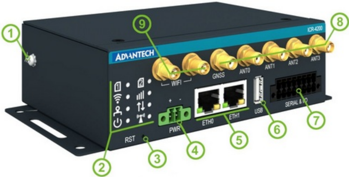
Figure 1: Router hardware overview – front view
