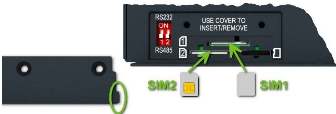
Figure 9: SIM Cards Insertion
