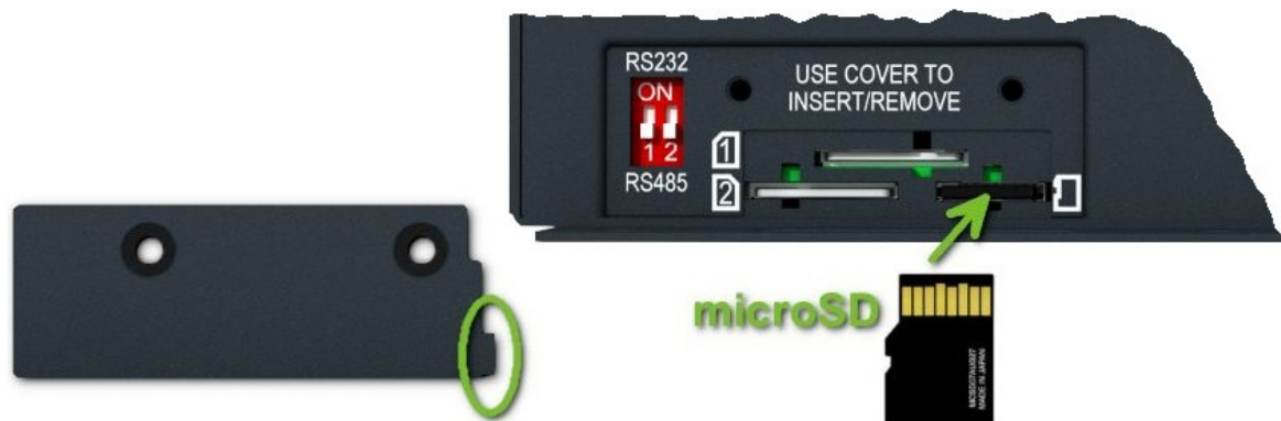
Figure 18: MicroSD Card Insertion
