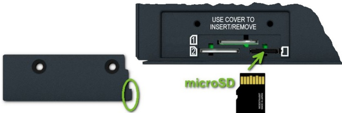
Figure 14: MicroSD Card Insertion
