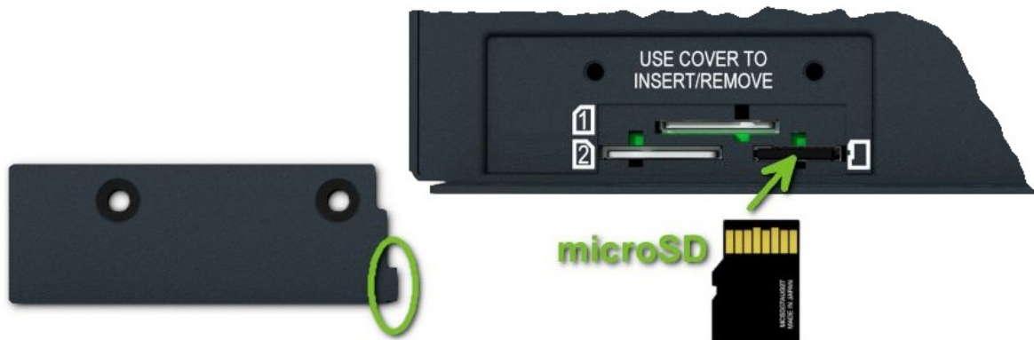
Figure 17: MicroSD Card Insertion
