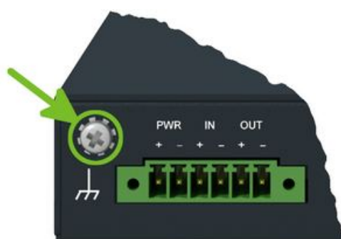
Figure 12: Position of the Grounding Screw
