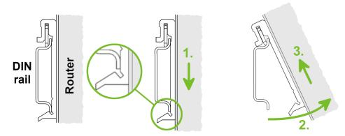
Figure 7: Removing Router from the DIN Rail
