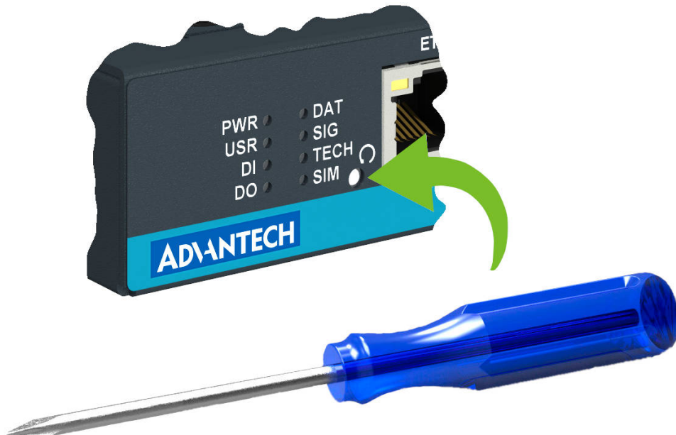
Figure 16: Resetting the Router
