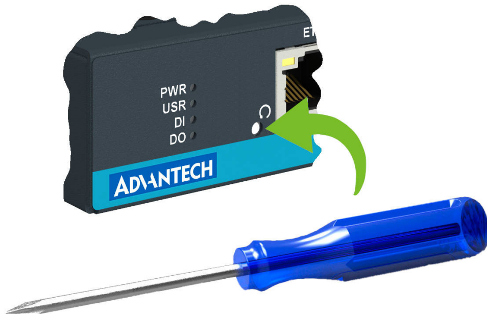
Figure 14: Resetting the router
