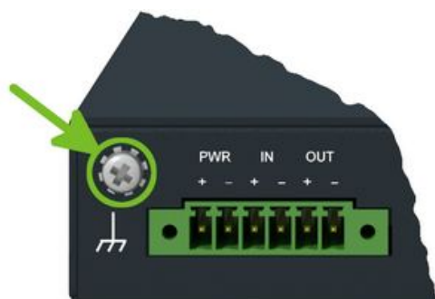
Figure 11: Grounding screw position
