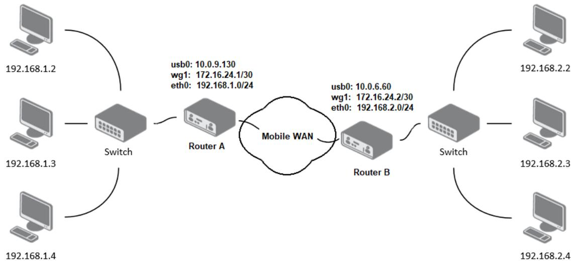
Figure 56: Topology of WireGuard Configuration Example
