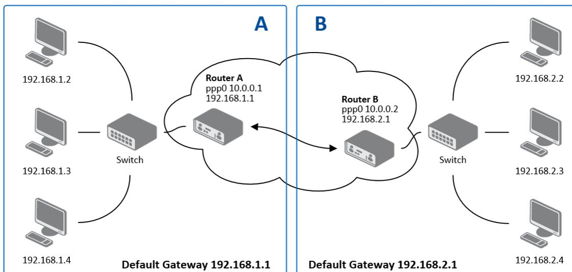
Figure 64: Topology of PPTP Tunnel Configuration Example
