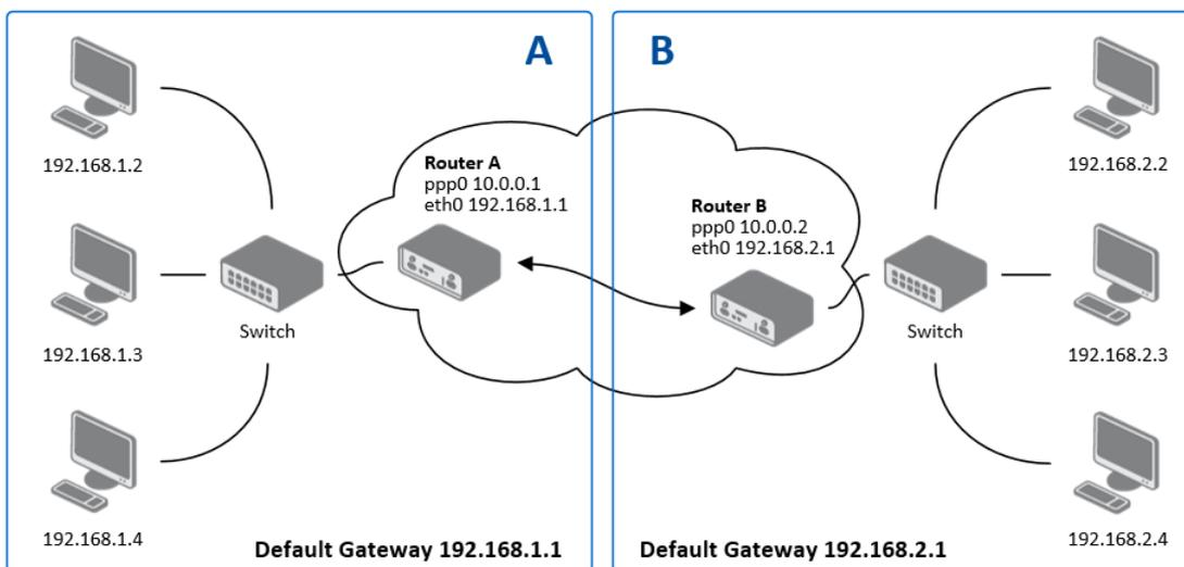
Figure 60: Topology of GRE Tunnel Configuration Example
