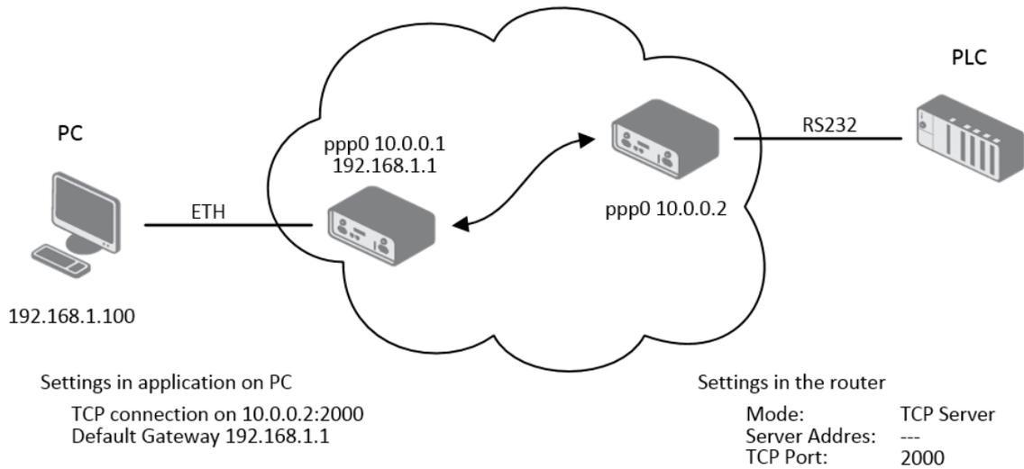
Figure 83: Example of Ethernet to serial communication configuration
