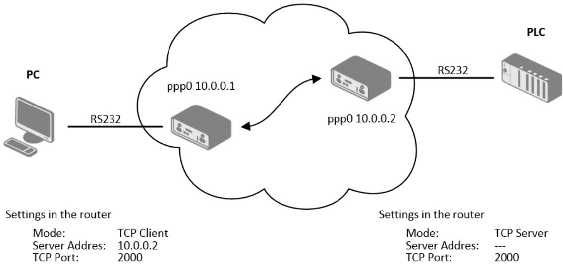
Figure 84: Example of serial interface configuration
