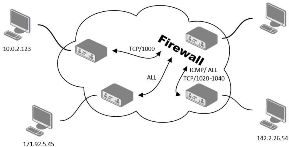
Figure 44: Topology for the IPv4 Firewall Configuration Example
