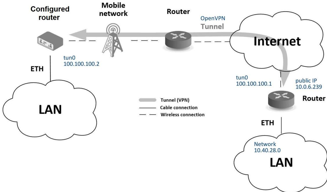
Figure 119: Secure networks interconnection – sample topology
