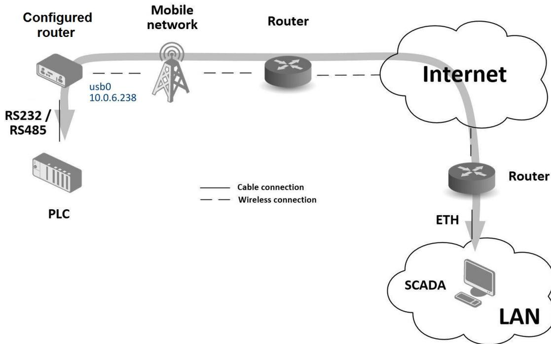
Figure 121: Serial Gateway – sample topology
