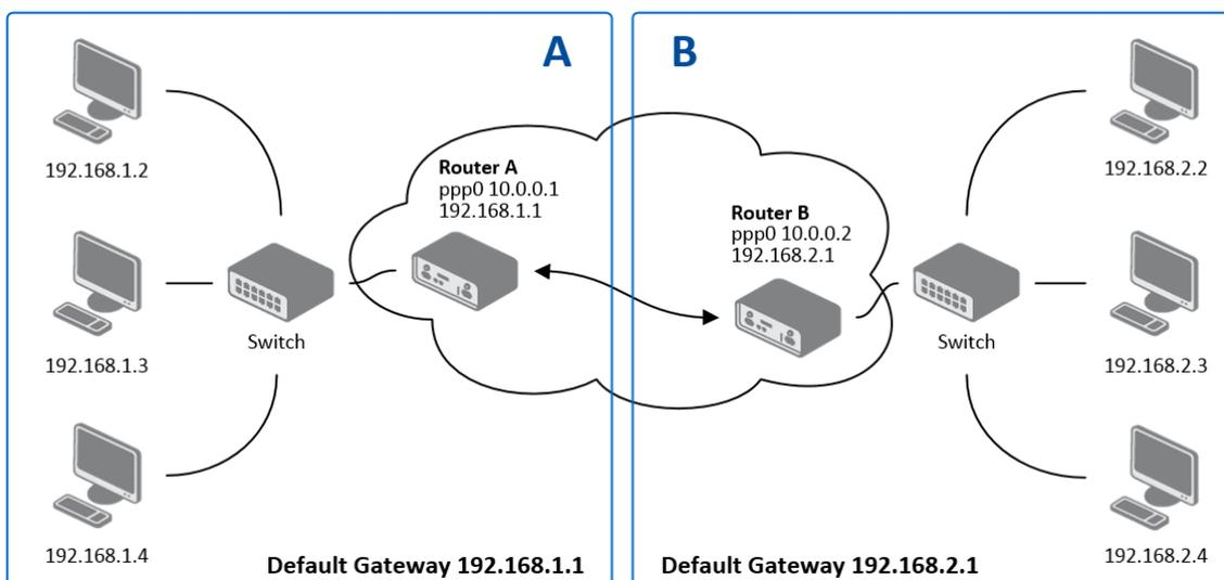
Figure 62: Topology of L2TP Tunnel Configuration Example
