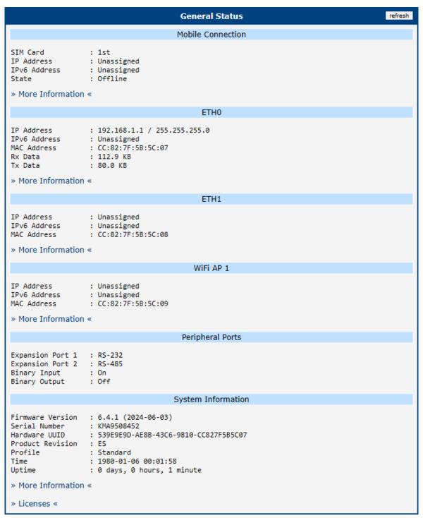
Figure 1: Web Configuration GUI
