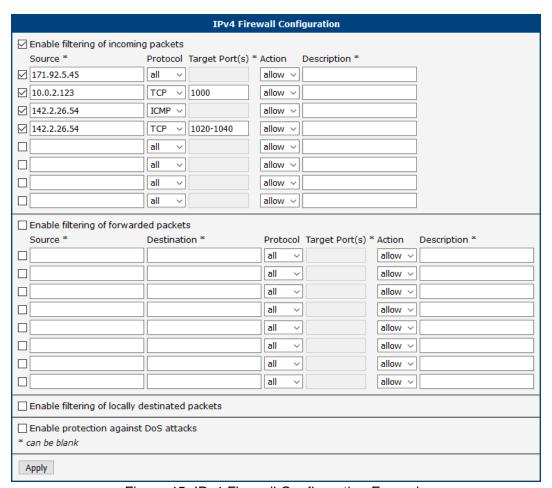
Figure 45: IPv4 Firewall Configuration Example
