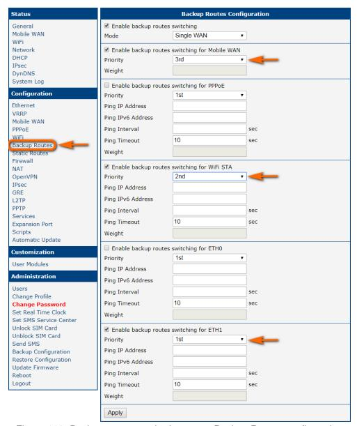
Figure 118: Backup access to the Internet – Backup Routes configuration
