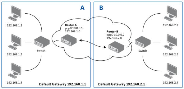
Figure 54: Topology of IPsec Configuration Example
