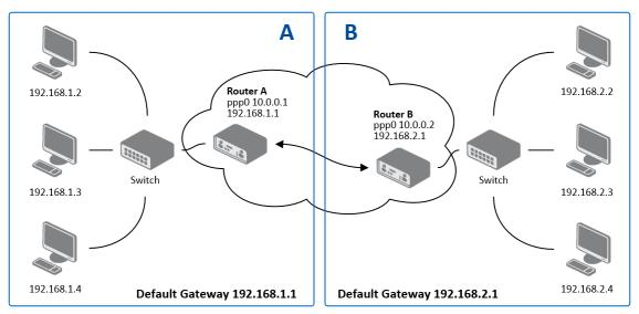
Figure 64: Topology of PPTP Tunnel Configuration Example
