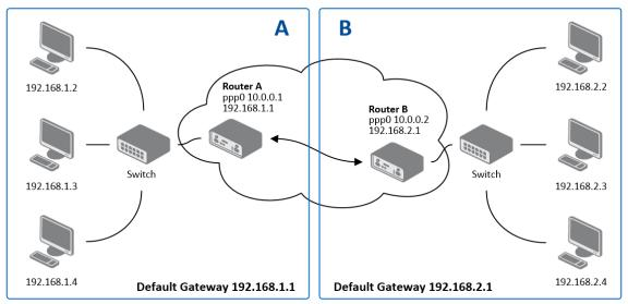
Figure 62: Topology of L2TP Tunnel Configuration Example
