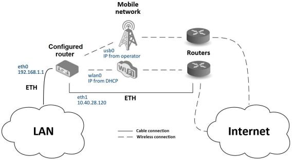
Figure 114: Backup access to the Internet - sample topology
