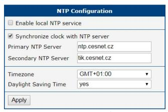
Figure 68: Example of NTP Configuration
