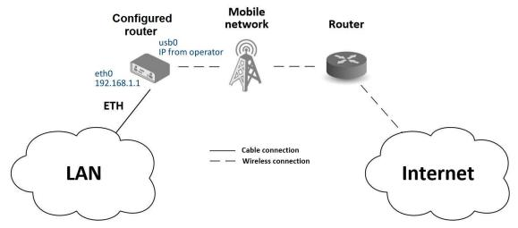
Figure 111: Access to the Internet from LAN – sample topology
