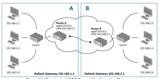
Figure 60: Topology of GRE Tunnel Configuration Example
