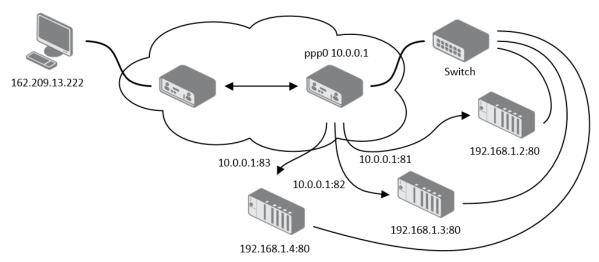
Figure 49: Topology for NAT Configuration Example 2
