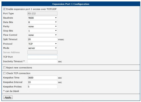
Figure 82: Expansion Port Configuration
