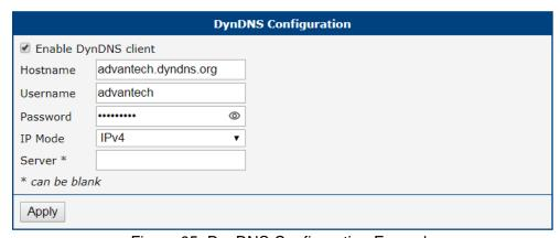
Figure 65: DynDNS Configuration Example
