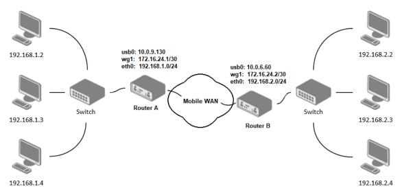
Figure 56: Topology of WireGuard Configuration Example
