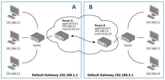
Figure 52: Topology of OpenVPN Configuration Example
