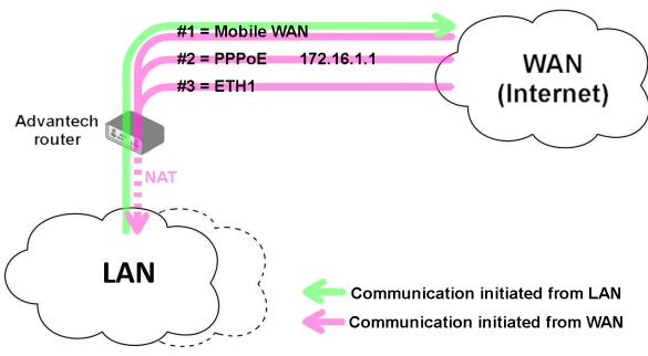
Figure 37: Example #3: Topology for Multiple WAN mode
