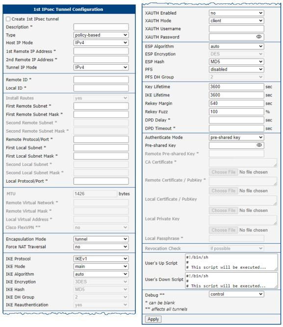
Figure 53: IPsec Tunnels Configuration Page
