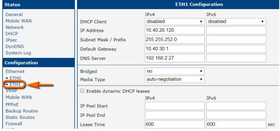
Figure 115: Backup access to the Internet – Ethernet configuration
