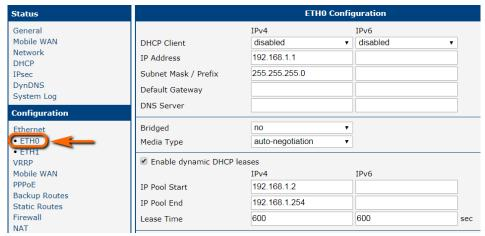
Figure 112: Access to the Internet from LAN – Ethernet configuration
