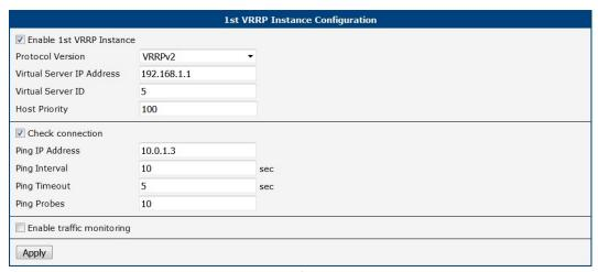
Figure 22: Example of VRRP Configuration – Backup Router
