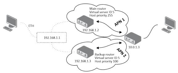
Figure 20: Topology of VRRP Configuration Example
