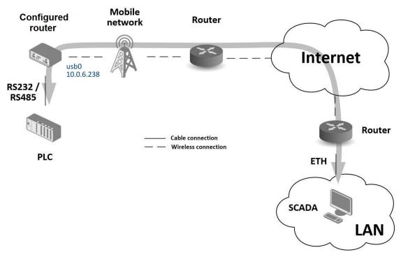
Figure 121: Serial Gateway - sample topology
