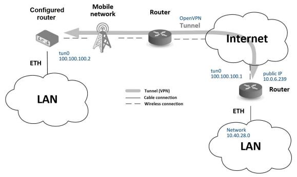
Figure 119: Secure networks interconnection – sample topology
