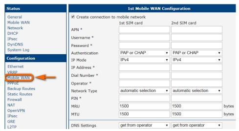
Figure 113: Access to the Internet from LAN – *Mobile WAN* configuration
