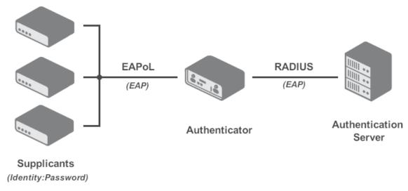
Figure 13: IEEE 802.1X Functional Diagram
