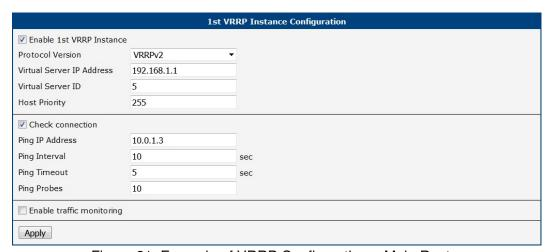
Figure 21: Example of VRRP Configuration - Main Router
