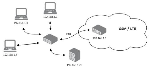
Figure 14: Network Topology for Example 1
