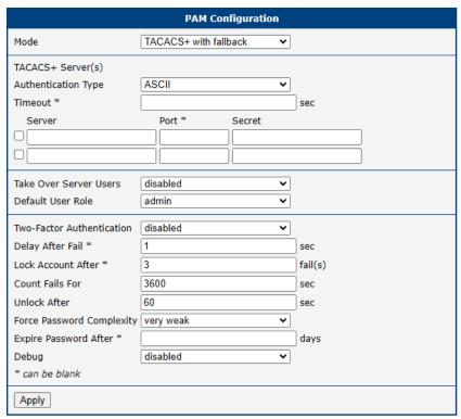
Figure 70: Configuration of TACACS+
