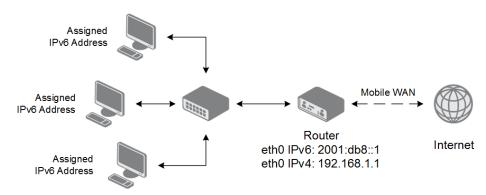
Figure 18: Network Topology for Example 3
