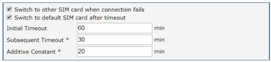
Figure 25: Configuration for SIM card switching Example 1
