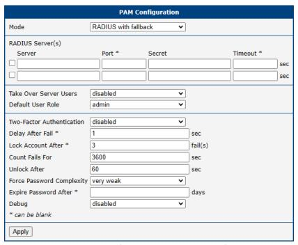
Figure 69: Configuration of RADIUS
