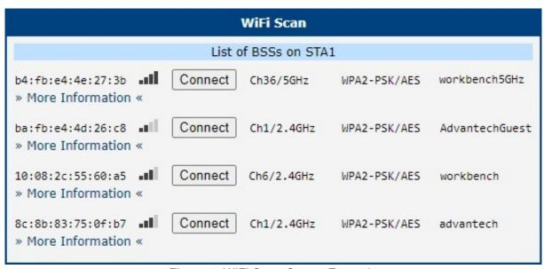
Figure 4: WiFi Scan Output Example
