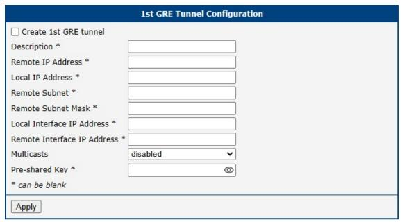
Figure 59: GRE Tunnel Configuration Page
