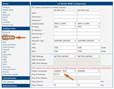
Figure 117: Backup access to the Internet – Mobile WAN configuration
