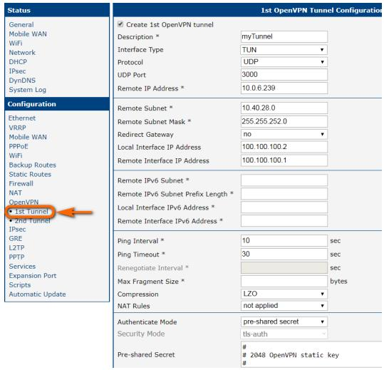
Figure 120: Secure networks interconnection – OpenVPN configuration
