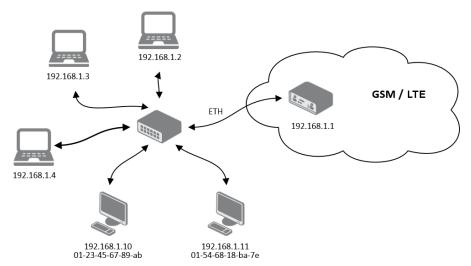
Figure 16: Network Topology for Example 2
