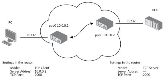
Figure 84: Example of serial interface configuration
