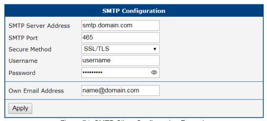
Figure 74: SMTP Client Configuration Example
