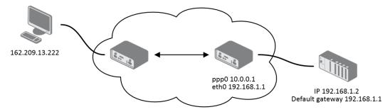
Figure 47: Topology for NAT Configuration Example 1
