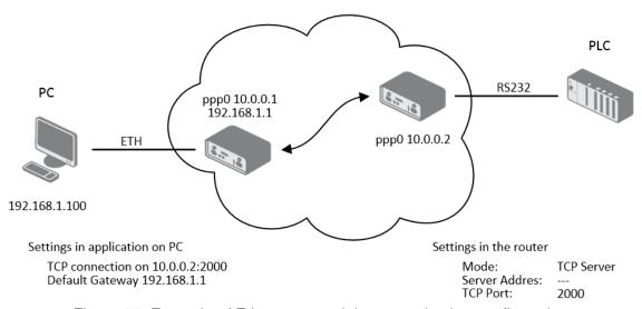
Figure 83: Example of Ethernet to serial communication configuration
