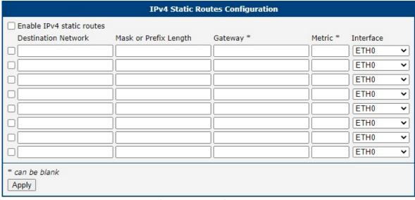
Figure 42: Static Routes Configuration Page
