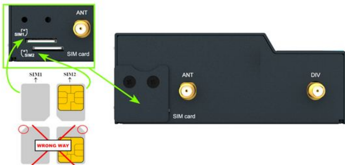
Figure 9: SIM card insertion
