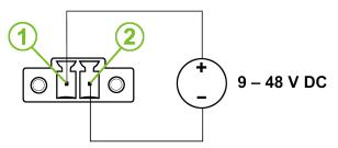
Figure 11: Power Connector Pinout
