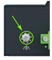
Figure 12: Position of the Grounding Screw
