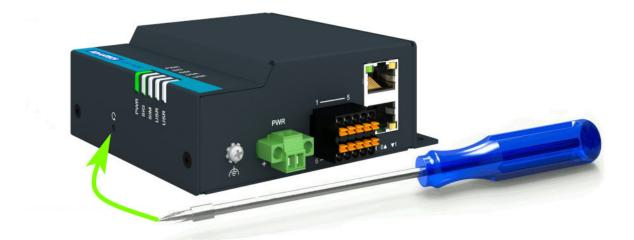
Figure 16: Resetting the Router
