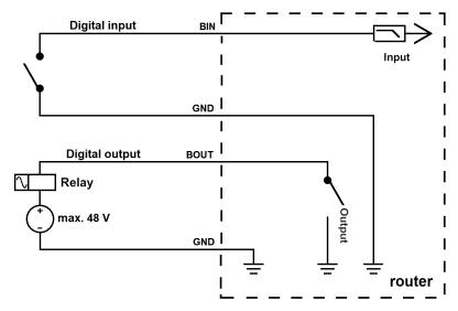
Figure 14: Functional Scheme of the Digital Interface
