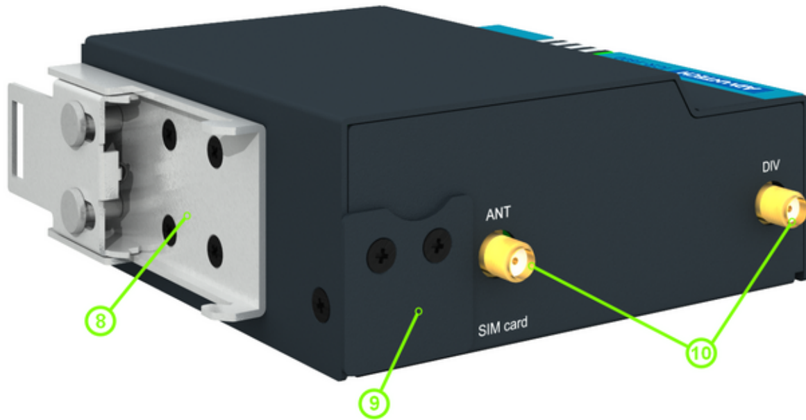
Figure 6: Router Hardware Overview: Rear View
