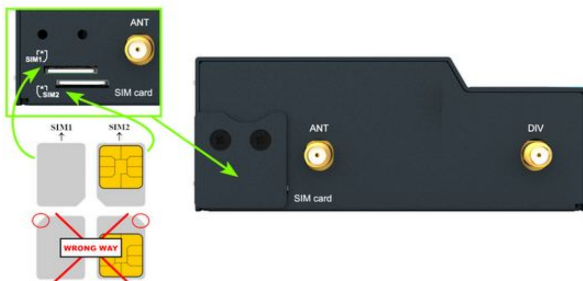
Figure 9: SIM card insertion
