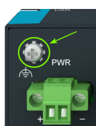
Figure 12: Grounding screw position
