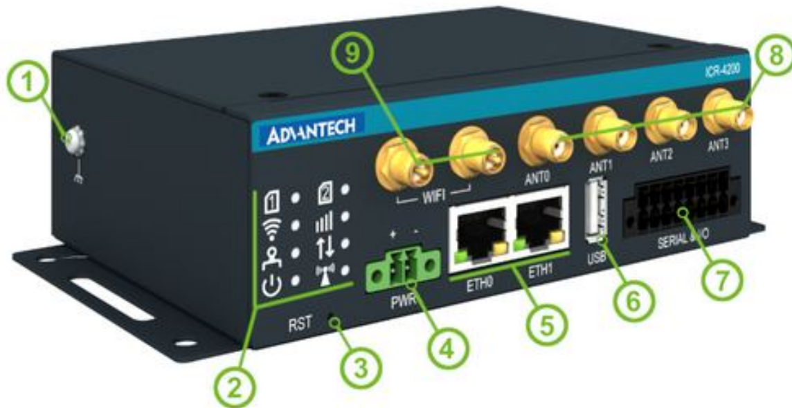
Figure 1: Router hardware overview – front view
