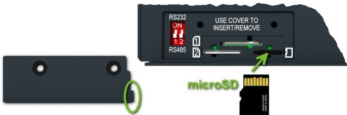
Figure 18: MicroSD Card Insertion
