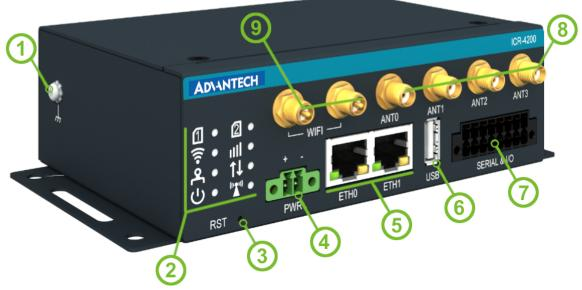
Figure 5: Router Hardware Overview: Front View
