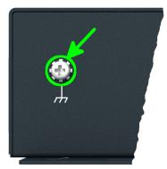
Figure 16: Position of the Grounding Screw
