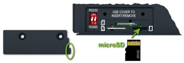
Figure 22: MicroSD Card Insertion
