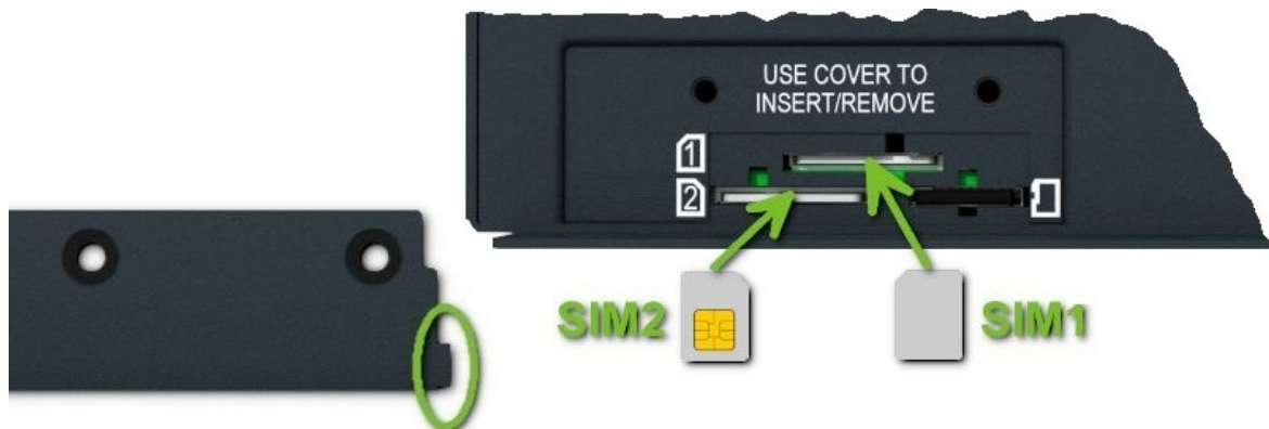
Figure 9: SIM Cards Insertion
