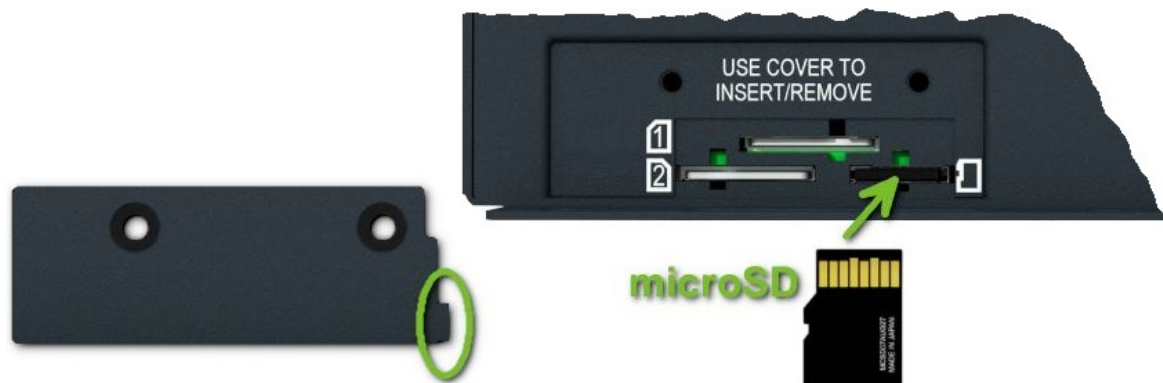
Figure 14: MicroSD Card Insertion
