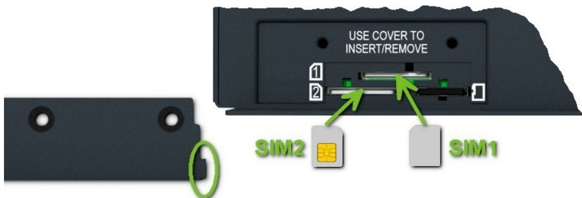
Figure 9: SIM Cards Insertion
