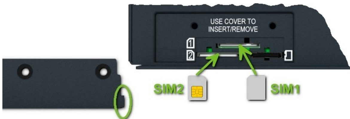
Figure 12: SIM Cards Insertion
