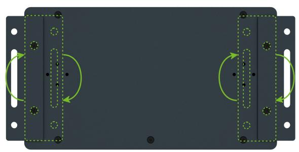
Figure 5: Rotated Wall Mounting Clips
