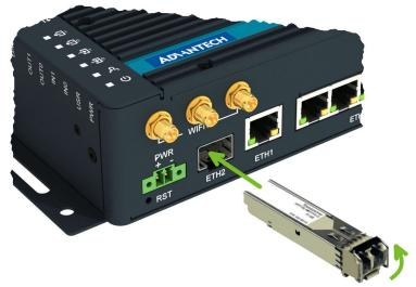
Figure 12: SFP Module Installation
