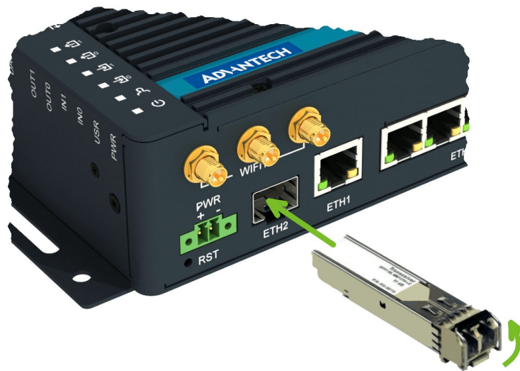
Figure 12: SFP Module Installation
