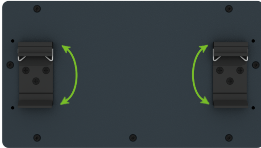
Figure 6: Default Position of the DIN Rail Clips
