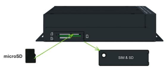
Figure 23: MicroSD Card Insertion
