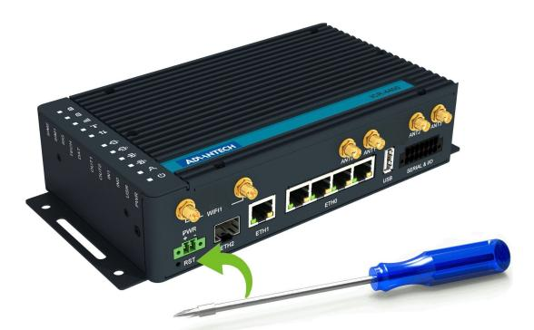
Figure 24: Resetting the Router
