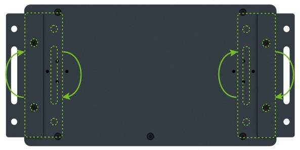
Figure 9: Rotated Wall Mounting Clips
