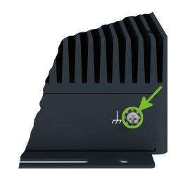
Figure 18: Position of the Grounding Screw
