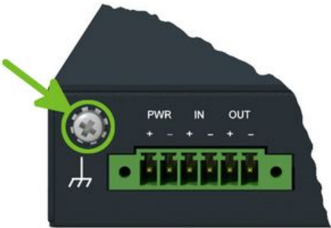
Figure 12: Grounding screw position
