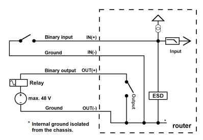
Figure 14: Functional Scheme of the Digital Interface
