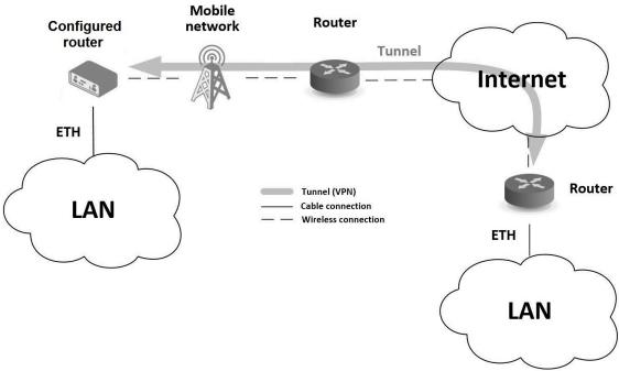
Figure 3: Using VPN Tunnel
