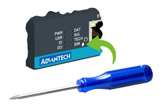
Figure 17: Resetting the Router
