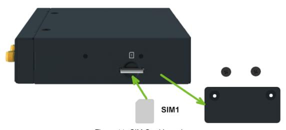
Figure 11: SIM Card Insertion
