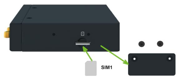
Figure 9: SIM Card Insertion
