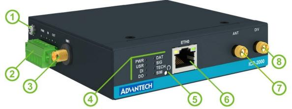
Figure 4: Router Hardware Overview: Front View
