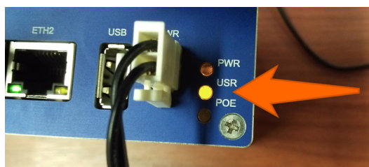
Figure 31: Example 1 – user LED turned on
