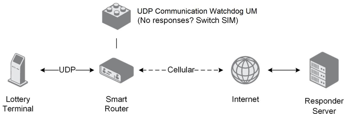
Figure 1: UDP Communication Watchdog operating principle
