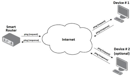
Figure 1: Functional Schema of Pinger Module
