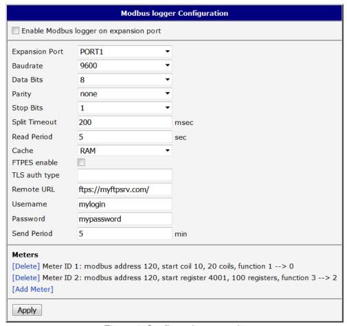
Figure 4: Configuration example
