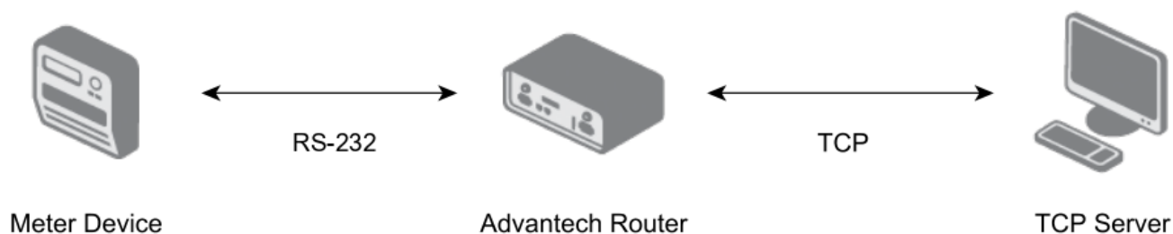
Figure 1: Serial to TCP router app function principle
